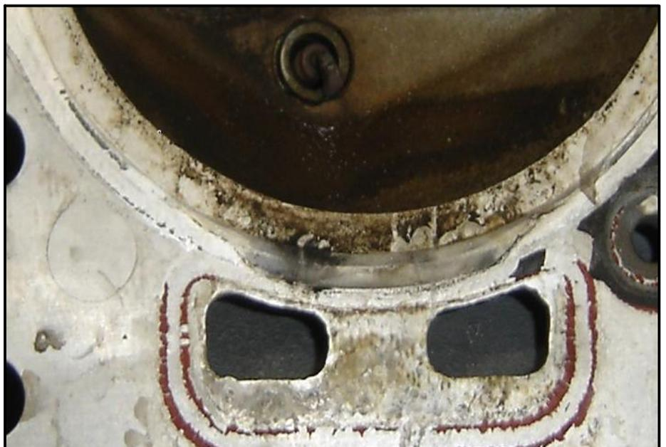
The system was once again pressure tested and seemed to hold just fine and not leak so I made an "educated guess" and suspected leaking head gaskets anyways. After removal of the heads the evidence was un-deniable. The A4 (right rear) cylinder had a spot on the head gasket combustion sealing ring that was leaking. Just a note, the head nuts were all tight (40 of them) and the car had never been overheated. It turns out that this problem is not un-common to this series of cars so be aware!
