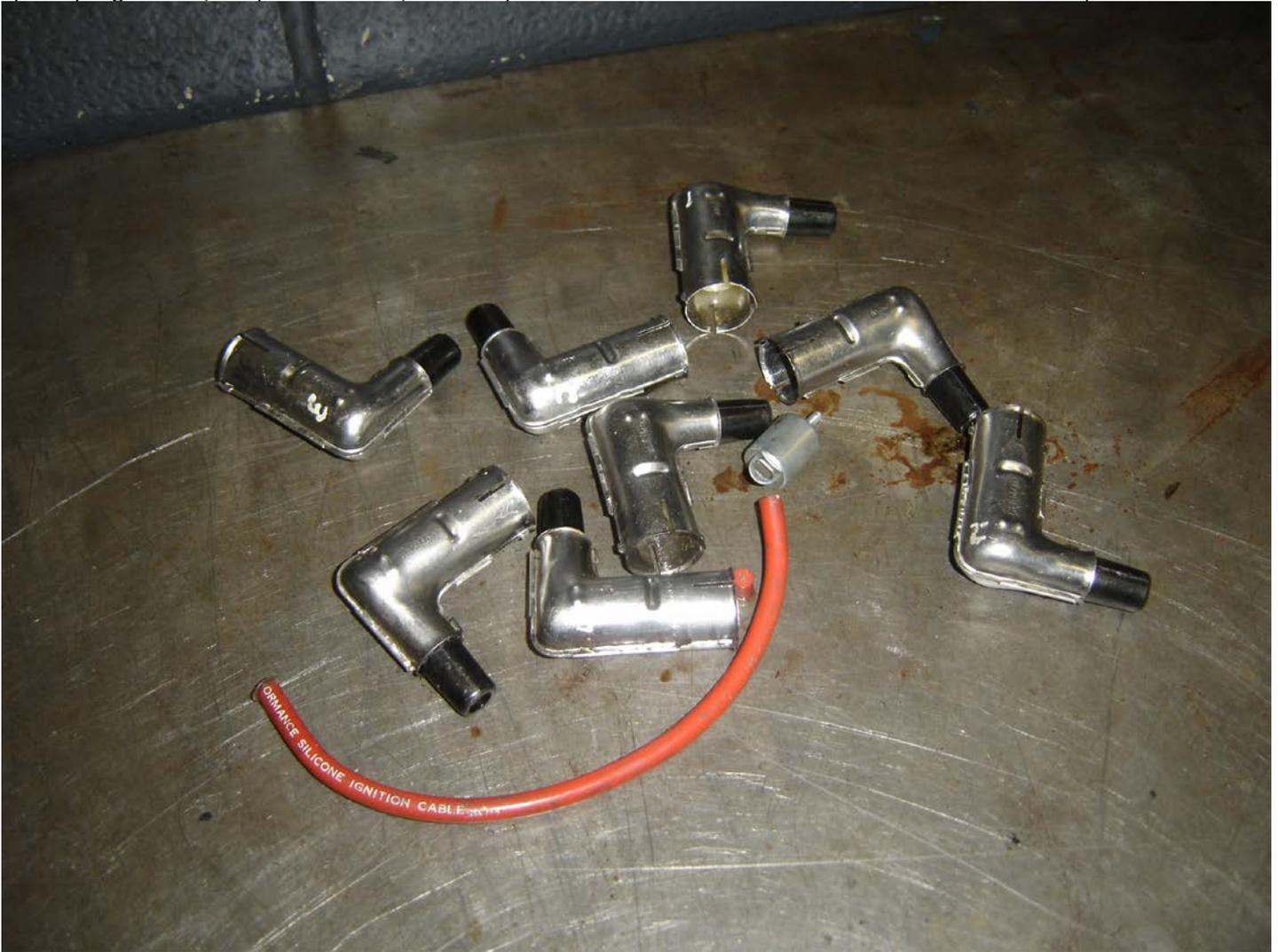
These metal cased wire ends are resistors which reduce static radio interference and are used with solid wire instead of resistor wire so I had to replace the coil wire with resistor wire to maintain the static reduction. During the next road test the car ran great, no more misfire under load and it restarted immediately when warm. Problem fixed!
